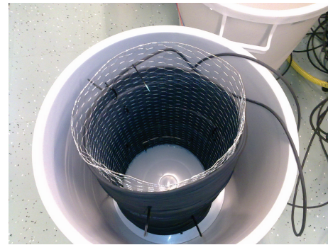
FIGURE 2: The cable was wrapped around a metal frame which was positioned inside the plastic tub.
