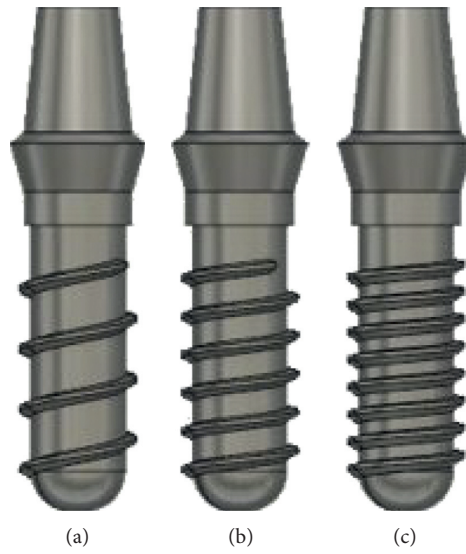
FIGURE 1: Configurations of implants with an abutment. (a) Single threaded 2.2 mm pitch. (b) Single threaded 1.4 mm pitch. (c) Single threaded 1 mm pitch.
