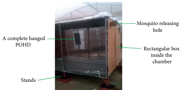
FIGURE 4: A bioassay box ( 187 \times 212 \times 115 cm) evaluating efficacy of POHD placed in the middle of a semifield chamber. The POHD is incorporated with different formulations of different synthetic attractive blends of different storage and usage period.
