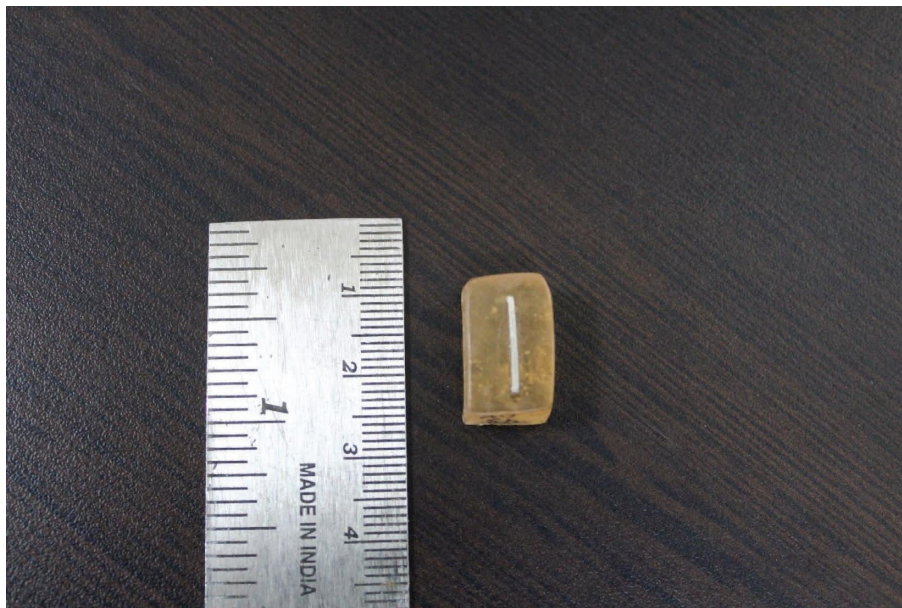
FIGURE 2: Samples embedded in polymethyl methacrylate resin.
