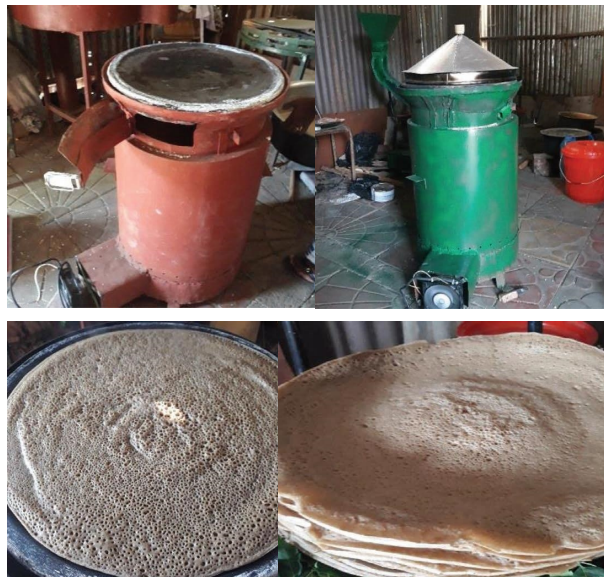
FIGURE 6: Prototype injera baking gasifier stove and texture of the produced injera.
