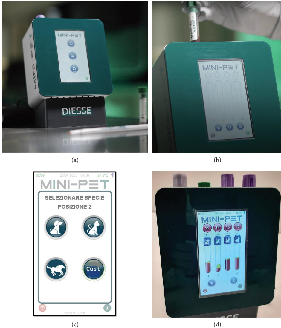
FIGURE 1: Picture representation of the use of the MINI-PET device for the ESR. (a) Appearance of MINI-PET for the ESR; (b) after the initialization, the blood tube has to be placed in one of the 4 channels of the device, and then the optical unit evaluates the level of the sample and starts the process of reading in a 14-minute countdown; (c) species selection; (d) after 14 minutes, the result is shown on the device display.
