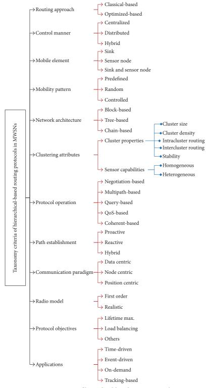
FIGURE 2: Taxonomy criteria of hierarchical-based routing protocols in MWSNs.
