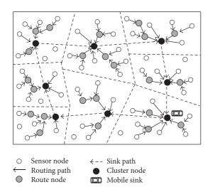
FIGURE 11: ABC-based data collection mechanism.
