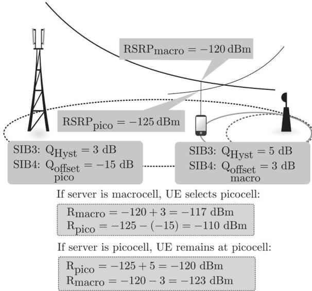
FIGURE 2: Illustration of the CRE for a UE in idle mode.
