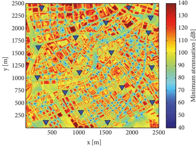
FIGURE 4: Minimum attenuation of the realistic scenario (Minimum attenuation for the complete (and not part of the) system area is represented. The path loss values correspond to both macro (triangles) and pico-cells (dots); hence this is the minimum net pathloss a UE would experience. 51 macros and 221 small cells are deployed in realistic case.).
