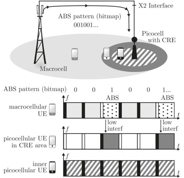
FIGURE 3: Illustration of how an LTE frame can consist of ABS subframes. Users in CRE area are only scheduled when the (time synchronized) macrocell transmits an ABS.
