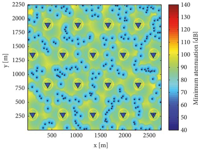
FIGURE 5: Minimum attenuation of the synthetic scenario (54 macros and 221 small cells are deployed in synthetic case.).
