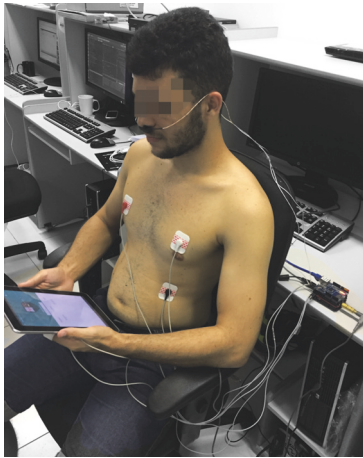
FIGURE 12: E-health shield collecting the patient's data.
