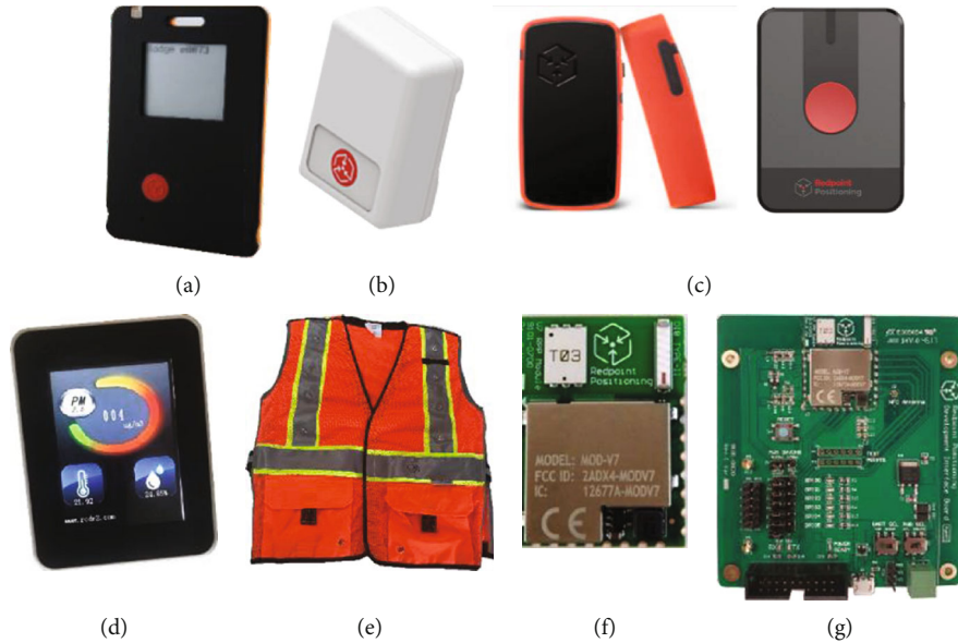
FIGURE 6: Seven common tags and units adopted in the proposed solution. (a) Badge tag. (b) Asset tag. (c) General tag. (d) Sensor tag. (e) Safety vest. (f) Positioning unit. (g) V7 development board.
