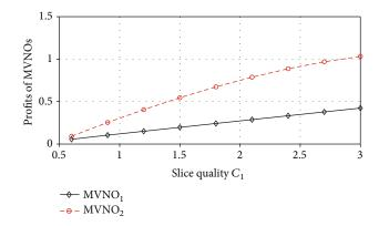
FIGURE 7: The profits of MVNO<sub>1</sub> and MVNO<sub>2</sub> versus slice quality  $C_1$  in the SG case.
