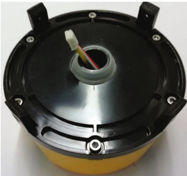
FIGURE 15: Structure diagram of the sealing method of Lezhi underwater robot.
