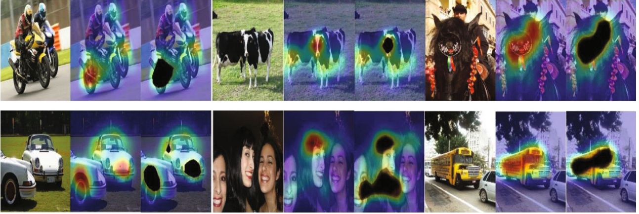
FIGURE 4: Selected examples of the discriminative object mined by weakly supervised object location and generate hard examples.
