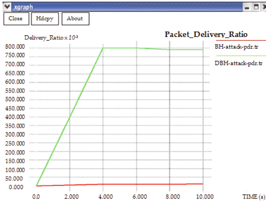
FIGURE 10: PDR with varying time for black hole and detected black hole attack.
