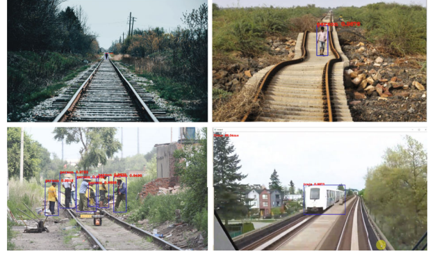
FIGURE 11: Object detection results. We used the open-source coco data set with 80 classes to train the model, and the images to be detected only include trains and people two classes.
