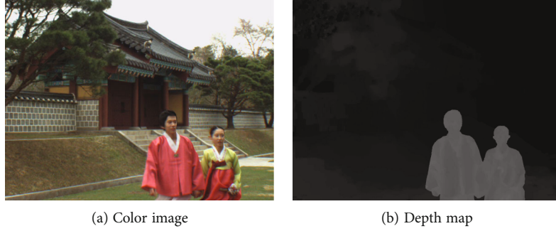
FIGURE 1: A sample image and its corresponding depth map from LoveBird1 MVD sequence: (a) synthesized image, view 8 frame 112, (b) corresponding depth image.
