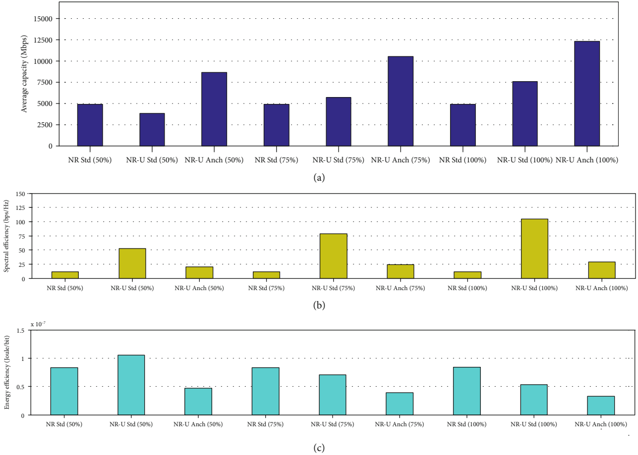
FIGURE 3: Average capacity, SE, and EE responses of small cells of a single operator of 5G NR standalone (Std), 5G NR-U Std, and 5G NR-U anchored (Anch) systems with the variation in its transmission time per FPP, including 50%, 75%, and 100% of FPP, which coexists with a single WiGig operator in a building for vRF = 1 and hRF = 1 . (a) average capacity, (b) SE, and (c) EE.
