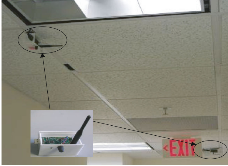
FIGURE 8: Example of the smart IoT environment and deployment of motion sensor devices are shown.
