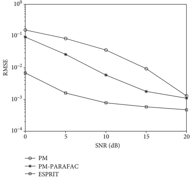
FIGURE 2: CFO performance comparison with different algorithms.
