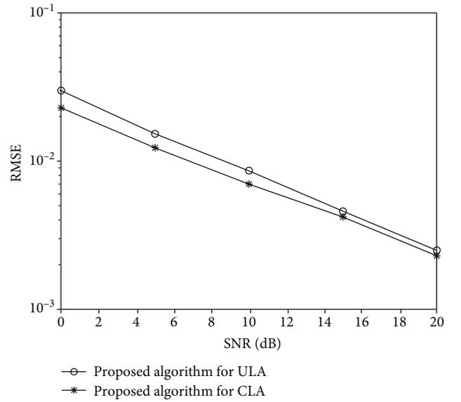
FIGURE 5: DOA performance comparison with different arrays.
