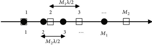
FIGURE 1: Coprime array structure model.
