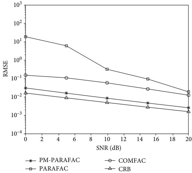
FIGURE 3: DOA performance comparison with different algorithms.
