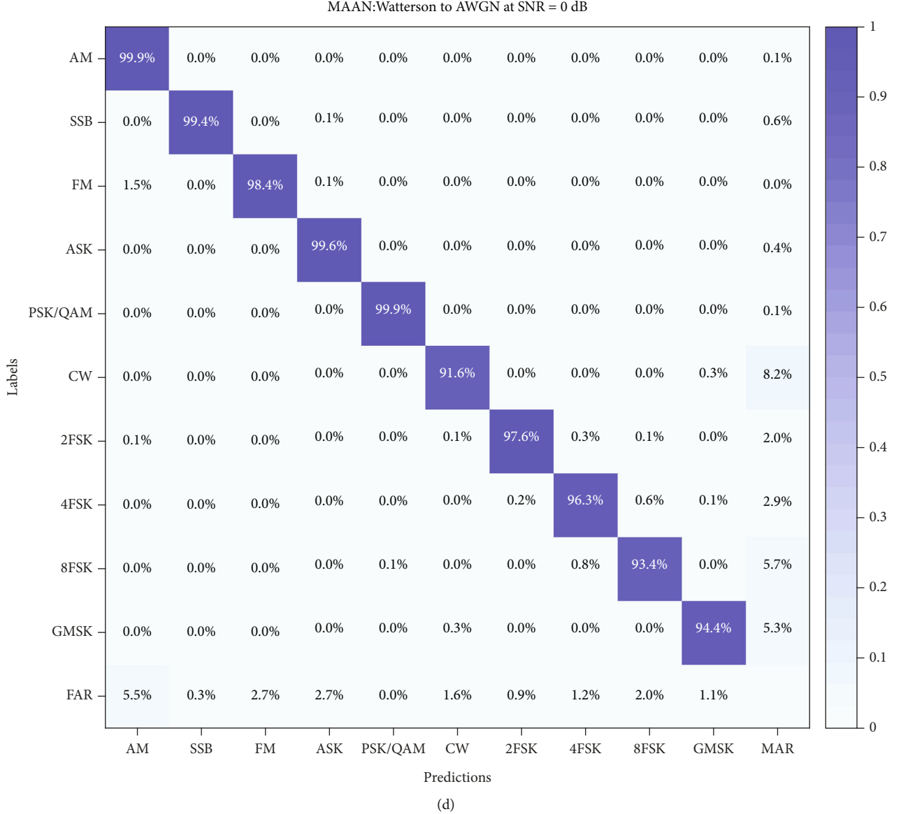
FIGURE 14: The performance of different methods in case 2. (a) The mAP vs SNR curves of different methods in an unknown environment. (b) The confusion matrix of the benchmark at SNR = 0 dB. (c) The confusion matrix of the MSDIN at SNR = 0 dB. (d) The confusion matrix of the MAAN at SNR = 0 dB.
