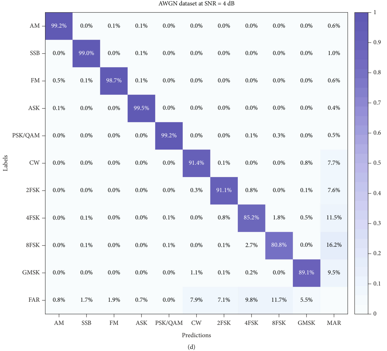
FIGURE 7: The performance of different methods on the AWGN dataset. (a) The mAP vs SNR curves of different methods. (b) The confusion matrix of MSDIN at SNR = 4 dB. (c) The confusion matrix of MSDIN at SNR = 0 dB. (d) The confusion matrix of MSDIN at SNR = -4 dB.
