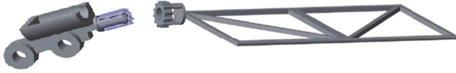
FIGURE 2: Wing angle adjustment mechanism.
