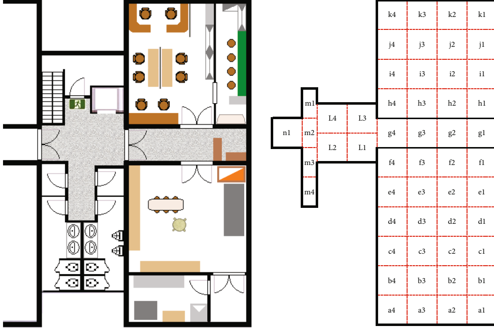
FIGURE 3: Measurement area of the ambient RF power and coordinates of all measurement positions.
