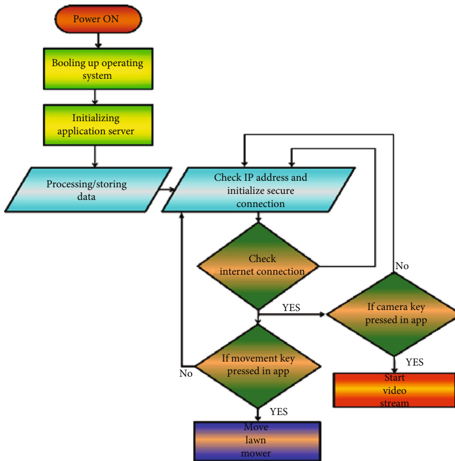
FIGURE 3: Local area server communication flowchart.
