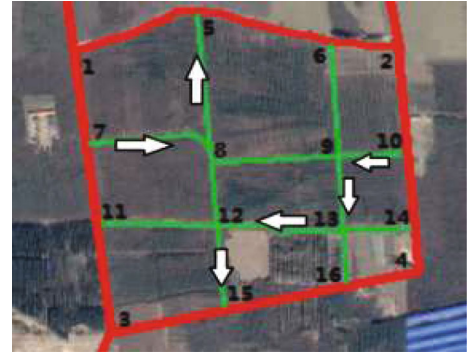
FIGURE 4: Optimization plan diagram (arrows indicate branch road sections with one-way diversion, and non-arrow main road sections are driven in both directions).
