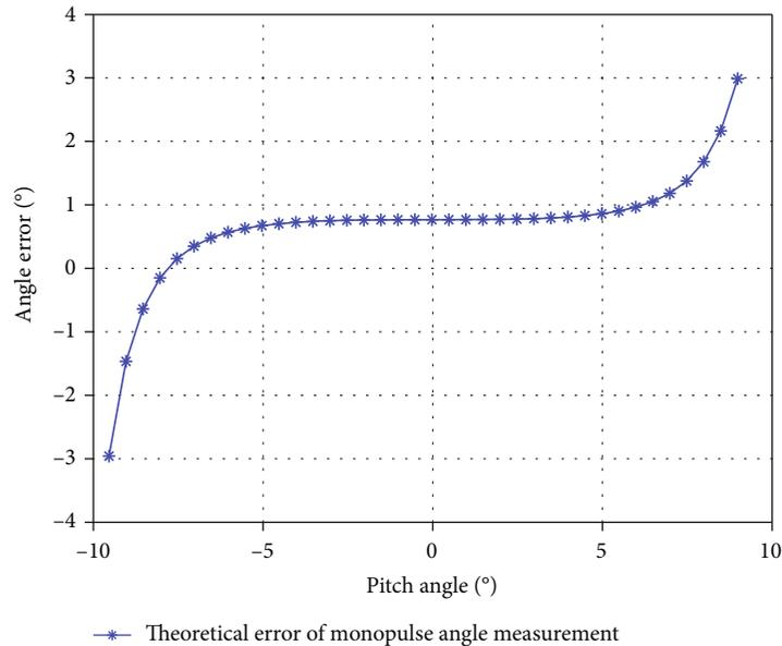
FIGURE 4: Mono-pulse angle tracking error curve based on beam pattern.
