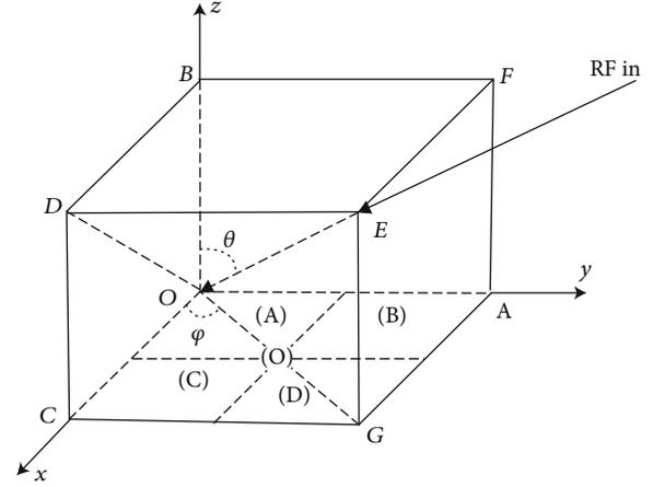
FIGURE 1: Angle measurement coordinate diagram of planar-phased array antenna.
