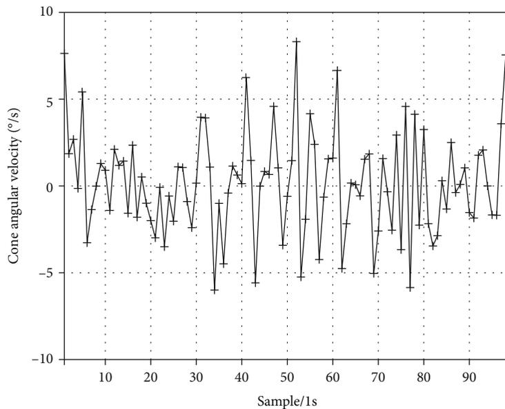
FIGURE 8: Large dynamic cone angular velocity (combination of azimuth and pitch angle).
