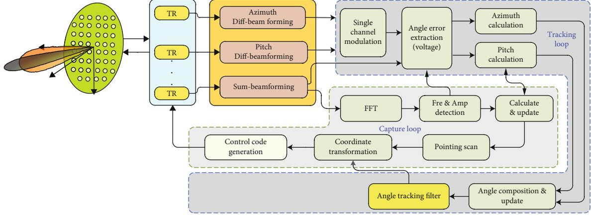
FIGURE 2: The block diagram of angle capture and tracking of the mono-pulse technology.
