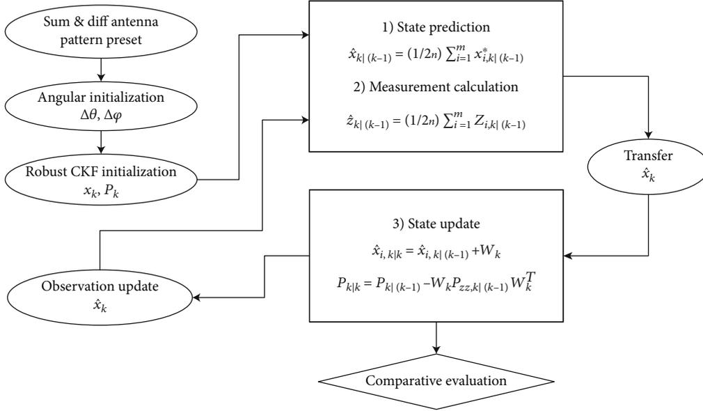
FIGURE 5: Simulation flow diagram.
