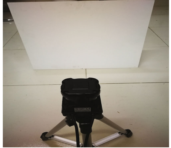
FIGURE 5: Intensity measurement at different sites in incident angle experiments: (a) intensity measurement at different sites of 0.1 m-14.4 m under the reference incident angle of 0^\circ ; (b) the picture of the scanning scene.
