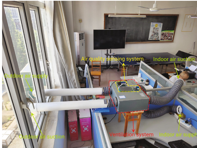
FIGURE 11: IoT prototype of IAQMCS system.
