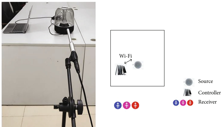
FIGURE 10: LOS acoustic signal production and acquisition. The principle of control variables should be obeyed in each experiment.
