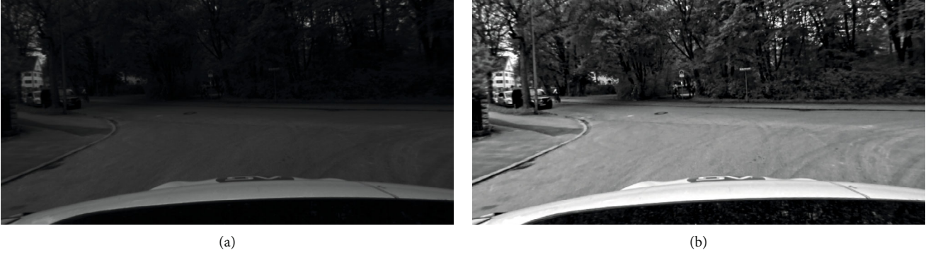
FIGURE 4: The low-light scene enhancement method. (a) The original image. (b) The enhanced image.
