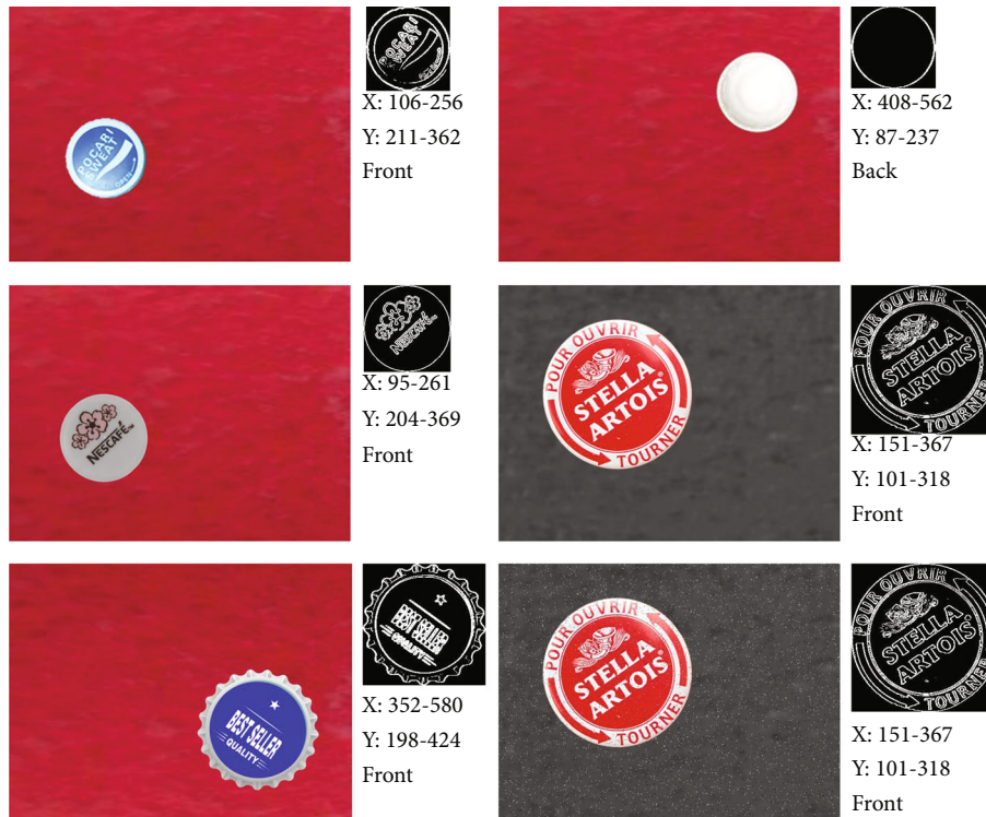
FIGURE 14: Comparison of the results of selecting different caps, conveyor belts, and sharpness.
