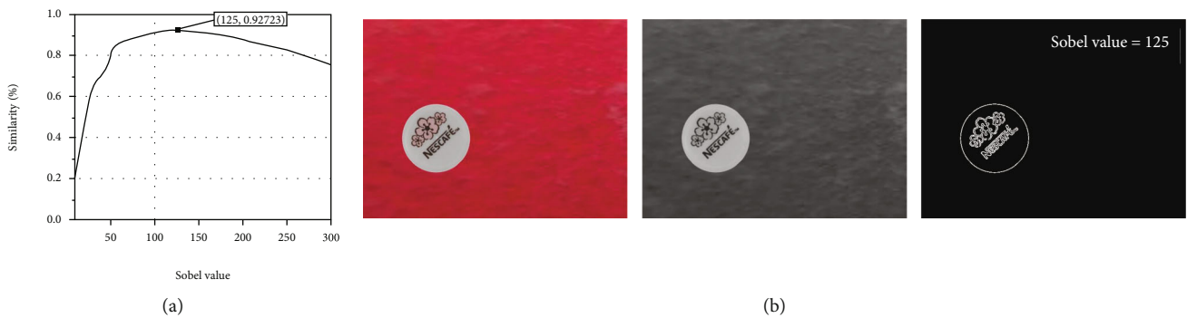
FIGURE 11: Sobel edge module results schematic. (a) The similarity between the images obtained with different thresholds and Ground Truth. (b) The original image and the image before and after the Sobel edge detection module.
