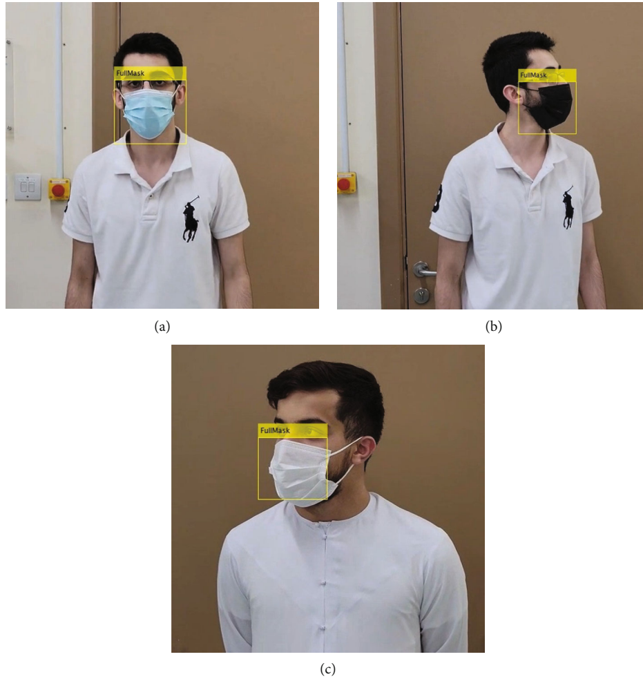
FIGURE 11: Full face mask classification using YOLOv2 object detection for a student wearing (a) blue mask and facing forward, (b) black mask and facing to the left, and (c) white mask and facing to the right.
