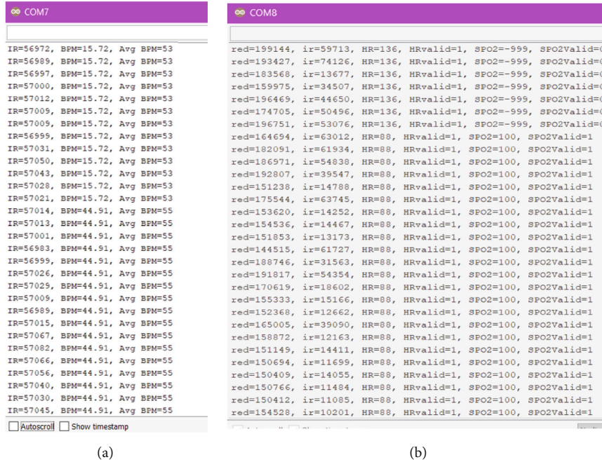
FIGURE 10: Output data (a) when applying knuckle onto the sensor instead of fingertip and (b) showing valid sensor output with accurate readings.
