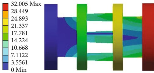
FIGURE 7: The shape of the first 4th-order splitting mode.
