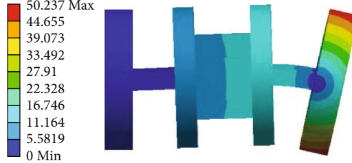
FIGURE 7: The shape of the first 4th-order splitting mode.
