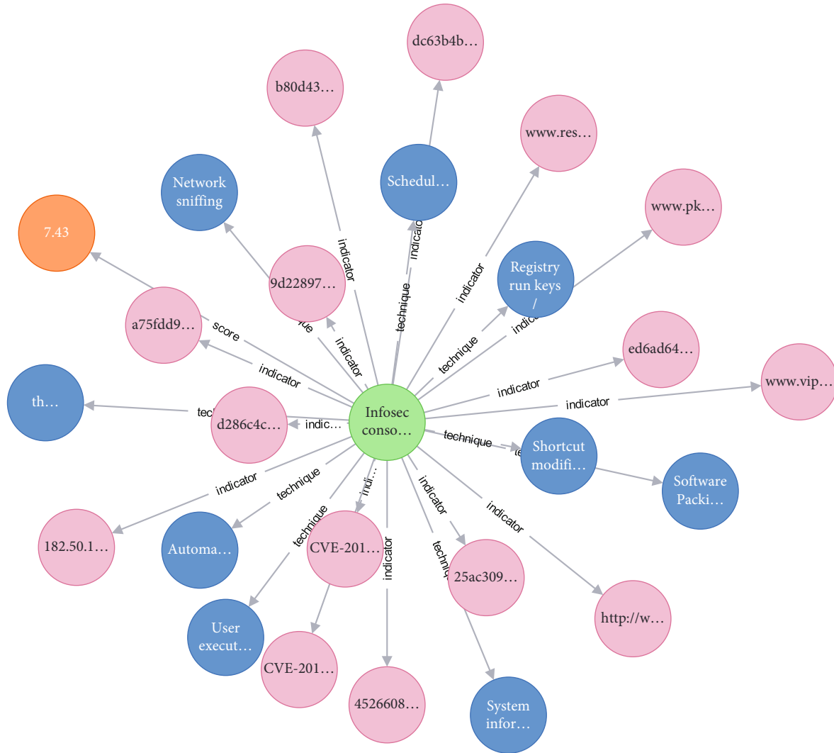
FIGURE 3: One threat intelligence scoring and visualization. Green circle represents threat reports, pink circles represent threat indicators, blue circles represent ATT&CK techniques, and yellow circle represents threat report quality scores.
