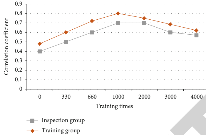
FIGURE 5: Correlation coefficients of training and test groups in the ANN model under different training times.
