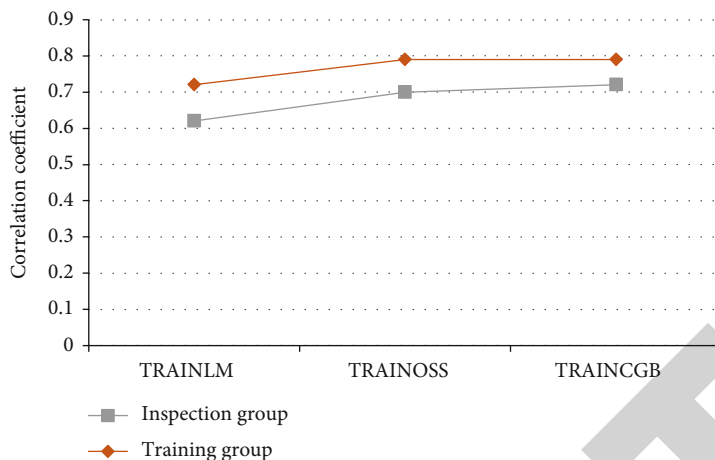
FIGURE 7: Correlation coefficients of training and testing groups in ANN models under different training functions.
