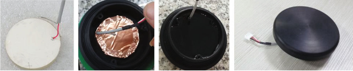
FIGURE 13: The customized sheet ceramic transducer.
