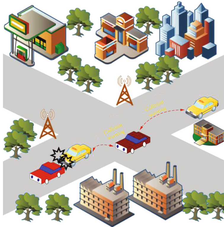
FIGURE 14: Collision Avoidance System (CAS) in Internet of Vehicles (IoV).
