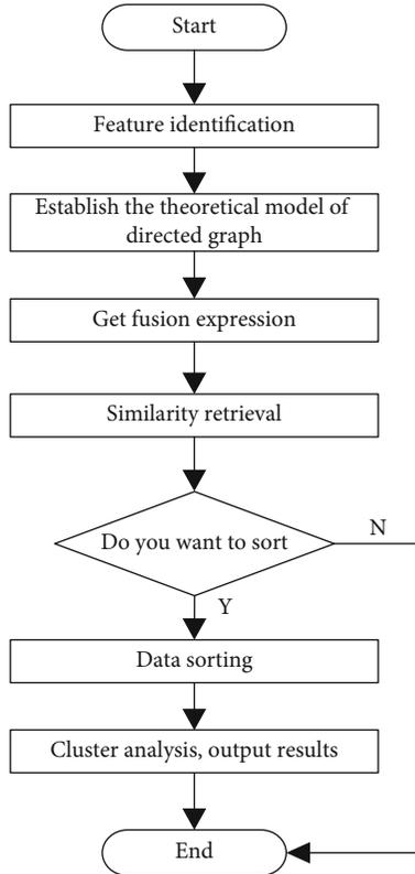
FIGURE 3: Flow chart of image retrieval of smart archives based on directed graph theory.
