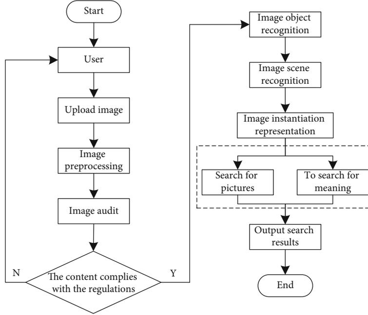
FIGURE 1: Workflow diagram of mobile visual retrieval service.
