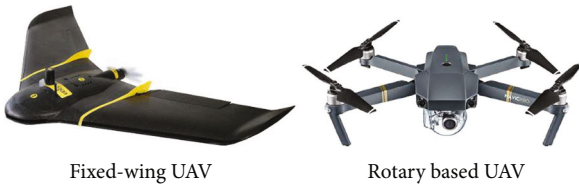
FIGURE 2: Two main types of UAVs.
