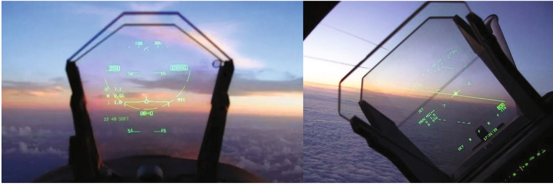
FIGURE 1: Key information enhancement of warplane based on a head-up display device.
